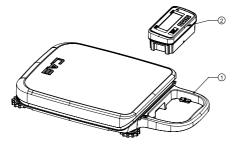
■ If you unscrew a bolt at Bracket handle(①), you can separate the indicator(②).
